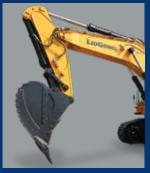
Breaking and lifting for 12 hours a day is an extreme workout for the boom, arm and hydraulics. So we've built-in extra strength and protection to keep these important components in peak condition. The super-strong boom design benefits from integrally forged front and rear supports.
