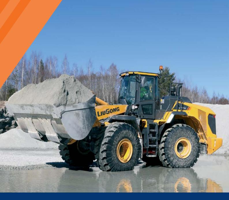
EngineCumminsNet Power286 hp (21Operating Weight24,500 kgBucket Capacity3.5 m³ – 7
